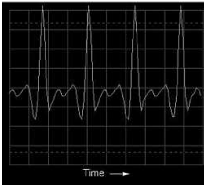
Figure 7.27: Oscilloscope display: waveshape of a trumpet tone.
