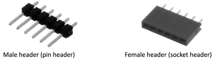
Figure 2.5 – Male header versus female header (image from https://en.wikipedia.org/wiki/Pin_header )
